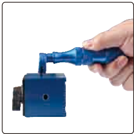
step 1: make grid cutting on surface
