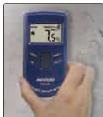
Measure concrete moisture
