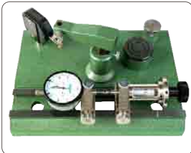
Inspect accuracy of dial indicators (range 0-25mm)
