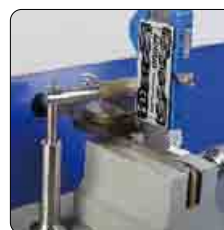
lapping measuring surfaces of caliper lower jaws
